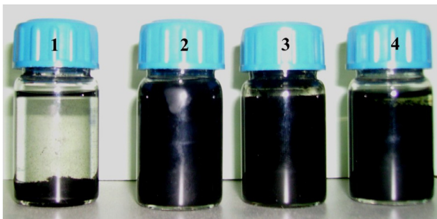
Fig. 1 – Pictures of the dispersion of the MWCNTs (0.2 g) in DMF (12 ml). 1-HCl-treated MWCNTs; 2-nitric acid-treated MWCNTs; 3-piranha treated MWCNTs; 4-MWCNTs after non-acidic treatment. Samples were kept for 100 days. MWCNTs were dispersed in DMF by sonication for 2 min.
